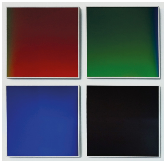
Figure 8: Photograph of the 56 x 57 cm 2 demonstrator modules with 4 different coating setups showing the colours red, green and blue; bottom right: uncoated glass.
