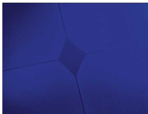
Figure 10: Close up photograph of blue demonstrator. Electrical cell interconnection is matching to backsheet in terms of colour. Only contours of solar cells are slightly visible from a few distinct viewing angles.
